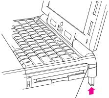
To lower the foot, press the rélease button. The foot extends automatically.
